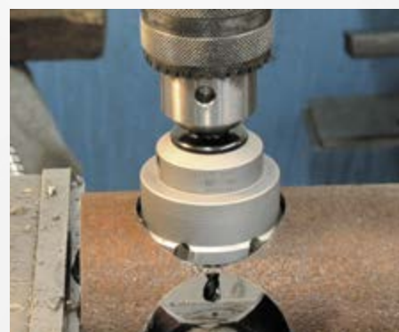
Bohren in Rohre
