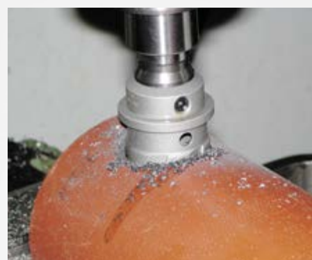
Bohren in Rohre
